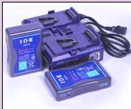
2 Endura Batteries and VL-2 Charger
