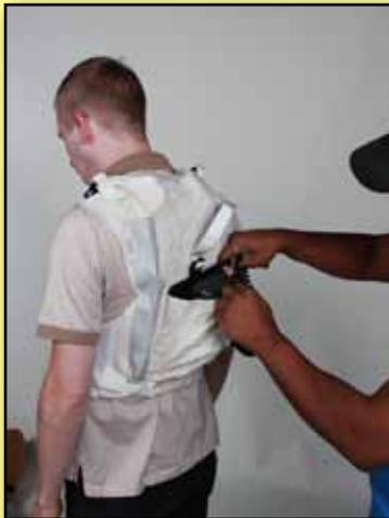
**3** Insert a fully charged Battery onto the V-Mount plate.
